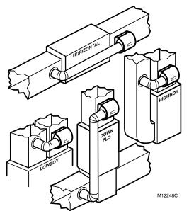
Fig. 3. Typical humidifier installation locations.
